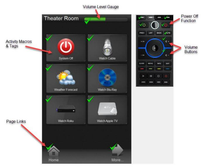
As referenced above, every controller in the system will use the same tag names. In the example of the volume gauge on top, since APEX does not tag this automatically, it is important to place the tags on it on every controller and room in the system file. The volume buttons, activity macros, page links and power off button will be tagged automatically by APEX, using the same naming convention throughout. This sets up for what is a powerful experience with the global controller.
