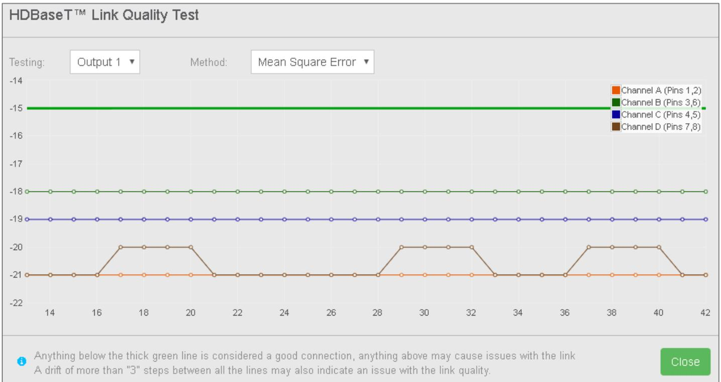
You may test each output, using the “Mean Square Error” one at a time. Anything below the green line is considered a good connection, and more than three steps between lines could indicate an issue with the quality of the link. A legend of each twisted pair that corresponds to the tests are indicated in the upper right. If there is a line above the green line or distance of more than 3 steps, re-terminating the cable or evaluation of the cable is in order.
