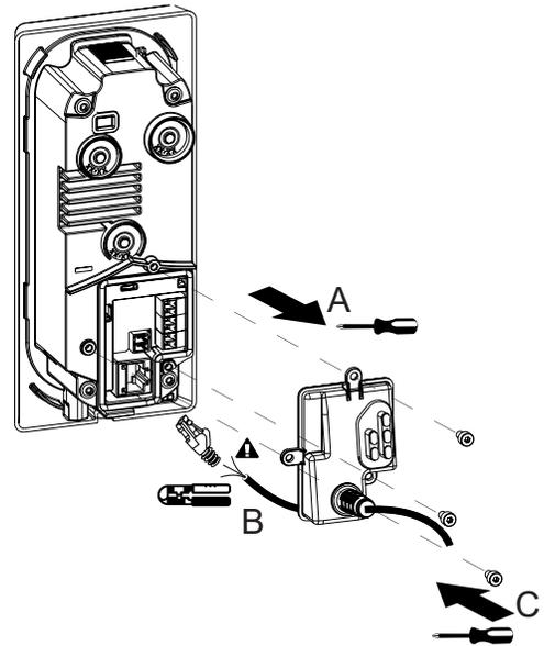
4. Put the main unit metal body in the surface mount box attached to the wall.
