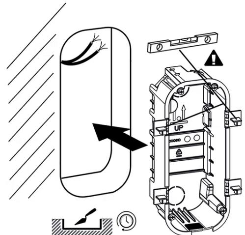
3. Use the four side bosses to determine the proper depth of the flush mounting. Make sure that the box edges are aligned with the wall after finishing the masonry. Break off the bosses after the walling material hardens.
