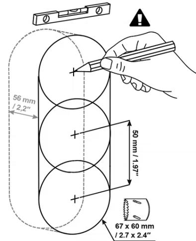
2. Remove one of the blinds on the plastic box and pull the cables through. The recommended length of the accessible cables is 15cm (22"). Mind the two arrows engraved on the box bottom and the included blind to keep the proper installation orientation. Place the box into the wall hole. Use the four side bosses to determine the proper depth of the flush mounting. Use walling material of your choice.
