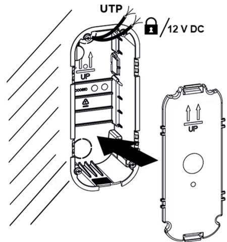
5. Let the walling material harden after finishing the masonry and wall surfacing and remove the blank.
