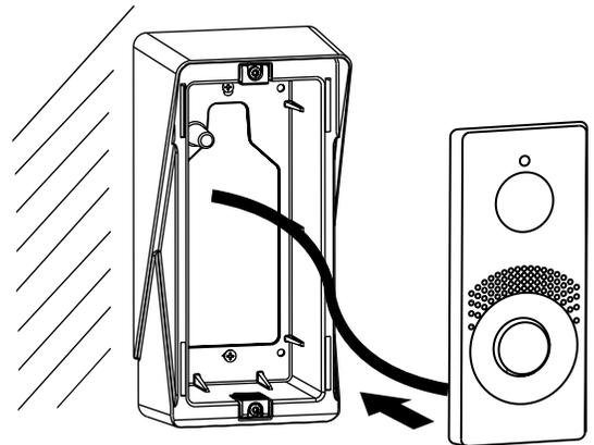
5. Press the main unit to the box and push it upwards. Screw a Torx head screw from the device bottom.
