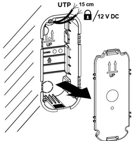
6. The package includes an L-shaped plastic plate and 3 Torx head screws. Cut 1–2mm (0.04-0.08") off the upper part of the cylinder-shaped rubber on the plate. Pull the cable through the remaining part. Use a crimping tool to crimp the cable connector and insert it in the terminal. Cover the terminal space with a plate and screw it.
