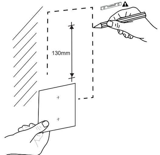
2. Put the surface mount box on the wall. Pull the available cables through the box opening. Fit the surface mount box using the included countersunk head screws.
