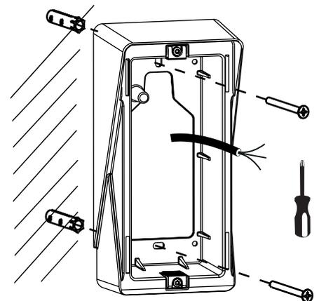
3. The main unit package includes an L-shaped plastic plate and 3 Torx head screws. Cut 1–2mm (0.04-0.08") off the upper part of the cylinder-shaped rubber on the plate. Pull the cable through the remaining part. Use a crimping tool to crimp the cable connector and insert it in the terminal. Cover the terminal space with a plate and screw it.
